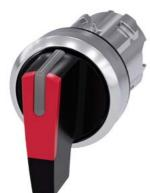
Selector switch, illuminable, 22 mm, round, metal, shiny, red, selector switch, long, 3 switch positions I>O<II, momentary contact type, actuating angle 2x45°, 10:30h/12h/13:30h, Z=50-unit packaging
