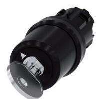
Key-operated switch BKS, 22 mm, round, plastic, Lock number E1 (VW), without key, 2 switch positions O-I, latching, actuating angle  $90^{\circ}$ , 10:30h/13:30h, key removal O, with laser labeling, lower case
