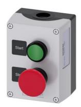
enclosure for command devices, 22 mm, round, enclosure material plastic, enclosure top part gray, 2 control points plastic, B=Pushbutton green, label: start, 1 NO, screw terminal, A=Mushroom pushbutton red, momentary contact type, label: Stop, 1 NC, screw terminal, floor mounting, 1xM20 each on top and bottom, Labels glued in
