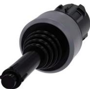
Coordinate switch, 22 mm, round, plastic with metal front ring, black, 4 switch positions, momentary contact type, with mechanical interlocking, with laser labeling, lower case
