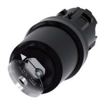
Key-operated switch IKON, 22 mm, round, plastic, lock number 360012K1, with 2 keys, 2 switch positions O<I, momentary contact type, Actuating angle 45°, 10:30h/12h, key removal O, with laser labeling, upper case and lower case, always upper case at the beginning of the word
