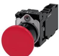
Mushroom pushbutton, 22 mm, round, plastic, red, 40mm, latching, pull-to-unlatch mechanism, with holder, 1 NO+1 NC, screw terminal, Z=20-unit packaging
