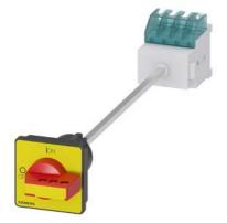
SENTRON, switch disconnector 3LD, EMERGENCY OFF switch, 3-pole, Iu: 16 A, Operating power / at AC-23 A at 400 V:  $7.5 \, \text{kW}$ , floor mounting with door coupling, defeatable knob-operated mechanism, red/yellow, 4-hole mounting of the handle
