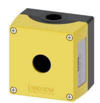
Enclosure for command devices, 22 mm, round, Enclosure material metal, Enclosure top part yellow, 1 control point, without equipment, Control point in center, floor mounting, 1xM20 each on top and bottom
