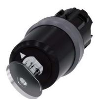
Key-operated switch BKS, 22 mm, round, plastic with metal front ring, Lock No. E7 (VW), without key, 2 switch positions O-I, latching, actuating angle 90°, 10:30h/13:30h, key removal O+I, Z=50-unit packaging
