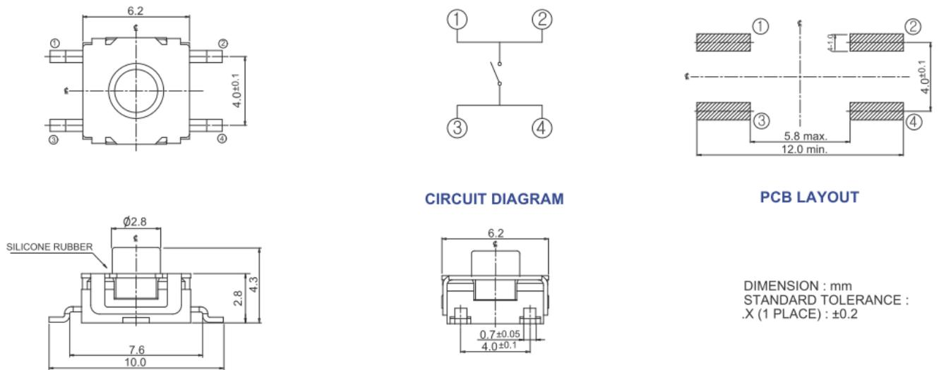
**Figure 2 – 222LJV, Surface Mount J Bend, Actuator Height 4.3mm**
