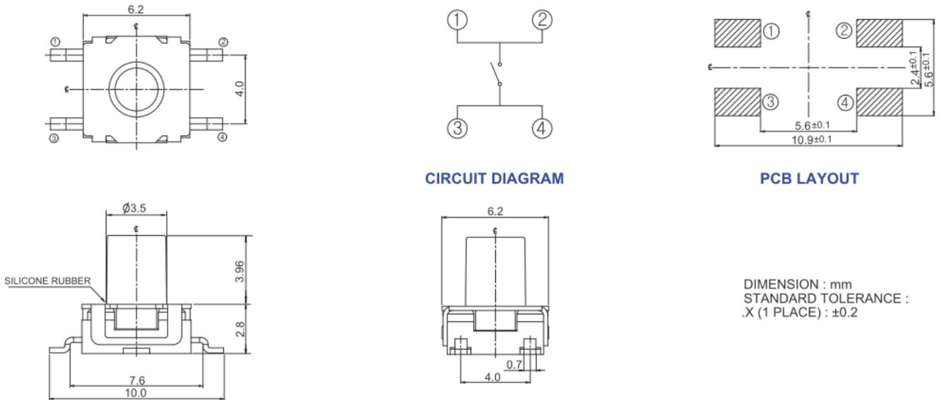
**Figure 2 – 222MJV..., Surface Mount J Bend, Actuator Height 6.8mm**
