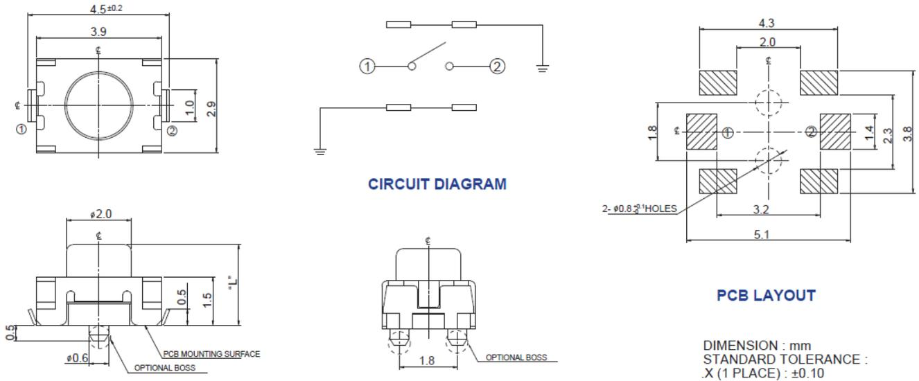
Figure 2 – 226HJ1VC..., Surface Mount J Bend Type1, With Flush Actuator
