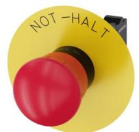
EMERGENCY STOP mushroom-type actuator, 22 mm, round, plastic, red, 40 mm, positive latching, according to EN ISO 13850, rotate-to-unlatch, with yellow backing plate, inscription: NOT-HALT, with holder, 1 NC, spring-type terminal, Z=20-unit packaging
