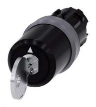
key-operated switch Siemens, 22 mm, round, plastic with metal front ring, lock number SSG10, with 2 keys, 3 switch positions I-O-II, latching, actuating angle 2x45°, 10:30h/12h/13:30h, key removal O+I, with laser labeling, inscription or symbol customer-specific selection with SIRIUS ACT configurator (CIN)
