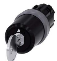
Key-operated switch BKS, 22 mm, round, plastic with metal front ring, lock No. E9 (VW), without key, 3 switch positions I-O-II, latching, actuating angle  $2x45^{\circ}$ , 10:30h/12h/13:30h, Key removal I+O+II, with laser labeling, upper case and lower case, always upper case at beginning of line
