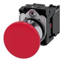
Mushroom pushbutton, 22 mm, round, metal, shiny, red, 40mm, latching, pull-to-unlatch mechanism, with holder, 1 NC, screw terminal, with laser labeling, lower case
