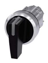
Illuminable selector switch, 22 mm, round, metal shiny, black, Selector switch long, 3 switch positions I-O<II, left latching, momentary contact type on the right, actuating angle 2x45°, 10:30 /12 /13:30, Z=50-unit packaging
