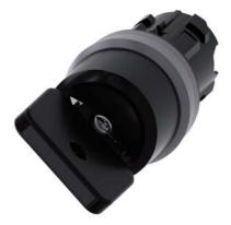
Key-operated switch O.M.R, 22 mm, round, plastic with metal front ring, lock number 73034, black, with 2 keys, 2 switch positions O-I, latching, actuating angle 90°, 10:30h/13:30h, key removal I, with laser labeling, upper case and lower case, always upper case at beginning of line
