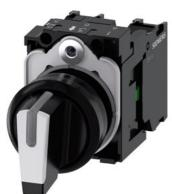
Selector switch, illuminable, 22 mm, round, plastic, white, selector switch, short, 3 switch positions |>O<|I|, momentary contact type, 10:30h/12h/13:30h, with holder, 1 NO, 1 NO, screw terminal, with laser labeling, inscription or symbol Customer-specific selection with SIRIUS ACT configurator (CIN)
