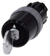
key-operated switch Siemens, 22 mm, round, plastic with metal front ring, lock number SSG10, with 2 keys, 3 switch positions I-O<II, left latching, momentary contact type on the right, actuating angle  $2x45^{\circ}$ , 10:30h/12h/13:30h, key removal I, with laser labeling, upper case and lower case, always upper case at the beginning of the word
