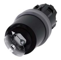
Key-operated switch IKON, 22 mm, round, plastic with metal front ring, lock number 360012K1, with 2 keys, 2 switch positions O<l, momentary contact type, Actuating angle  $45^\circ, 10:30h/12h,$  key removal O, with laser labeling, upper case and lower case, always upper case at beginning of line
