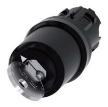
Key-operated switch IKON, 22 mm, round, plastic, special lock, with 2 keys, 2 switch positions O<I, momentary contact type, Actuating angle 45°, 10:30h/12h, Key removal O
