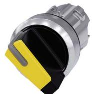
Selector switch, illuminable, 22 mm, round, metal, shiny, yellow, selector switch, short, 2 switch positions O<I, momentary contact type, Actuating angle 45°, 10:30h/12h, Z=50-unit packaging
