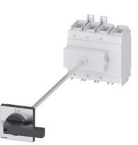
SENTRON, Switch disconnector 3LD, main switch, 4-pole, lu=250 A, Operating power / at AC-23 A at 400 V: 132 kW, floor mounting with door coupling, knob-operated mechanism, black, 4-hole mounting of the handle
