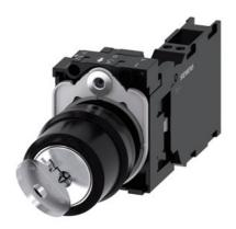
RONIS key-operated switch, 22 mm, round, plastic, lock number SB30, with 2 keys, 2 switch positions O-I, latching, 10:30h/13:30h, key removal O+I, with holder, 1 NO+1 NC, spring-type terminal, possible special locks: SB31, 421, 455, with laser labeling, inscription or symbol Customer-specific selection with SIRIUS ACT configurator (CIN)
