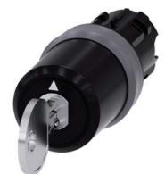
key-operated switch Siemens, 22 mm, round, plastic with metal front ring, lock number SSG10, with 2 keys, 3 switch positions I-O<II, left latching, momentary contact type on the right, actuating angle  $2x45^\circ$ , 10:30h/12h/13:30h, key removal I, with laser labeling, upper case and lower case, always upper case at beginning of line
