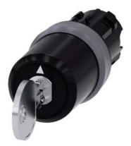
Key-operated switch BKS, 22 mm, round, plastic with metal front ring, lock number S1, with 2 keys, 3 switch positions I-O-II, latching, actuating angle  $2x45^{\circ}$ , 10:30h/12h/13:30h, Key removal I+O+II, with laser labeling, lower case
