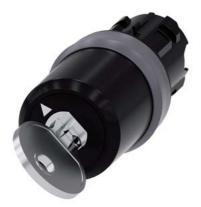
key-operated switch Siemens, 22 mm, round, plastic with metal front ring, lock no. LSG1, with 2 keys, 2 switch positions O-I, latching, actuating angle 90°, 10:30h/13:30h, key removal O, with laser labeling, upper case and lower case, always upper case at the beginning of the word
