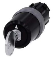
Key-operated switch BKS, 22 mm, round, plastic with metal front ring, lock number S1, with 2 keys, 3 switch positions I-O<II, left latching, right momentary contact type, actuating angle  $2x45^{\circ}$ , 10:30h/12h/13:30h, Key removal I
