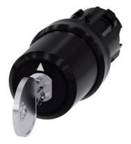
Key-operated switch BKS, 22 mm, round, plastic, Lock No. E2 (VW), without key, 3 switch positions I-O-II, latching, actuating angle 2x45°, 10:30h/12h/13:30h, Key removal I+O+II
