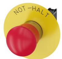
EMERGENCY STOP mushroom-type actuator, 22 mm, round, metal, shiny, red, 40 mm, positive latching, according to EN ISO 13850, rotate-to-unlatch, with yellow backing plate, inscription: NOT-HALT, with holder, 1 NC, screw terminal
