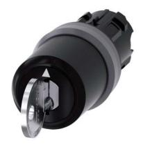
Key-operated switch IKON, 22 mm, round, plastic with metal front ring, lock number 360012K1, with 2 keys, 3 switch positions I-O-II, latching, actuating angle 2x45°, 10:30h/12h/13:30h, key removal O, with laser labeling, inscription or symbol Customer-specific selection with SIRIUS ACT configurator (CIN)
