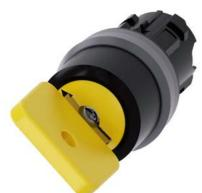
Key-operated switch O.M.R, 22 mm, round, plastic with metal front ring, lock number 73033, yellow, with 2 keys, 2 switch positions O<I, momentary contact type, Actuating angle 45°, 10:30h/12h, key removal O, with laser labeling, lower case
