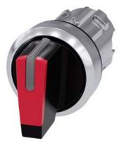
Selector switch, illuminable, 22 mm, round, metal, shiny, red, selector switch, short, 3 switch positions I-O<II, left latching, right momentary contact type, actuating angle  $2x45^{\circ}$ , 10:30h/12h/13:30h
