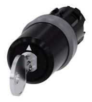
key-operated switch Siemens, 22 mm, round, plastic with metal front ring, lock number SSG10, with 2 keys, 3 switch positions I-O-II, latching, actuating angle 2x45°, 10:30h/12h/13:30h, key removal I+II, with laser labeling, upper case and lower case, always upper case at the beginning of the word
