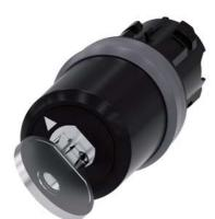
Key-operated switch BKS, 22 mm, round, plastic with metal front ring, Lock No. E2 (VW), without key, 2 switch positions O-I, latching, actuating angle 90°, 10:30h/13:30h, key removal O+I, with laser labeling, upper case
