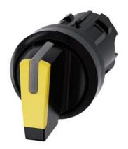
Selector switch, illuminable, 22 mm, round, plastic, yellow, selector switch, short, 3 switch positions >0<II, momentary contact on the left, latching on the right, actuating angle  $2x45^\circ$ , 10:30h/12h/13:30h, with laser labeling, upper case and lower case, always upper case at the beginning of the word
