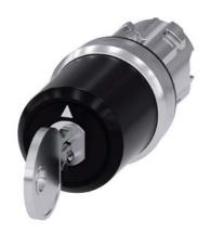
key-operated switch Siemens, 22 mm, round, metal, shiny, lock no. STGH10, with 2 keys, 3 switch positions I>O<II, momentary contact type, actuating angle  $2x45^\circ$ , 10:30h/12h/13:30h, key removal O, with laser labeling, upper case
