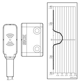
Safe switch on distance  $S_{ao}\ 6\ mm$
