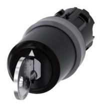
Key-operated switch IKON, 22 mm, round, plastic with metal front ring, lock number 360012K1, with 2 keys, 3 switch positions I-O<II, left latching, right momentary contact type, actuating angle  $2x45^{\circ}$ , 10:30h/12h/13:30h, key removal O+I, with laser labeling, lower case
