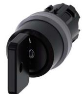
Key-operated switch O.M.R, 22 mm, round, plastic with metal front ring, lock number 73034, black, with 2 keys, 3 switch positions I-O<II, left latching, right momentary contact type, actuating angle 2x45°, 10:30h/12h/13:30h, key removal I, with laser labeling, upper case and lower case, always upper case at the beginning of the word
