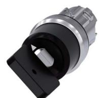
key-operated switch Siemens, 22 mm, round, metal, shiny, lock no. VL5, with 2 keys, 2 switch positions O-I, latching, actuating angle 90°, 10:30h/13:30h, key removal O, with laser labeling, inscription or symbol customer-specific selection with SIRIUS ACT configurator (CIN)
