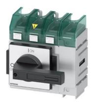
SENTRON, Molded case switch 3LD5 UL, Main switch, 4-pole, certified according to UL489 UL60947-4-1 and IEC60947-3, UL: 150A, SCCR 50kA at 480VAC, Operating power at 480VAC 3-phase: 100hp, IEC: 160A, Operating power at AC-23A at 400V: 75kW, floor mounting with direct handle, black, incl. terminal covers for the infeed side
