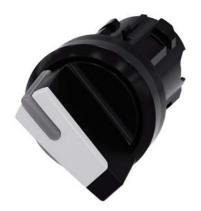
Selector switch, illuminable, 22 mm, round, plastic, white, selector switch, short, 2 switch positions O<I, momentary contact type, Actuating angle 45°, 10:30h/12h, with laser labeling, upper case and lower case, always upper case at beginning of line
