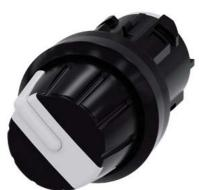
Selector switch, 22 mm, round, plastic, white, Rotary knob, 4 switch positions I-II-III-IV, latching, Actuating angle 4x90°, 3h/6h/9h/12h, with laser labeling, upper case and lower case, always upper case at the beginning of the word
