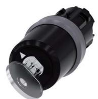
Key-operated switch BKS, 22 mm, round, plastic with metal front ring, lock number S1, with 2 keys, 2 switch positions O<I, momentary contact type, Actuating angle 45°, 10:30h/12h, key removal O, with laser labeling, lower case
