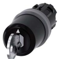
Key-operated switch IKON, 22 mm, round, plastic with metal front ring, lock number 360012K1, with 2 keys, 3 switch positions I>O<II, momentary contact type, actuating angle 2x45°, 10:30h/12h/13:30h, key removal O, Z=50-unit packaging
