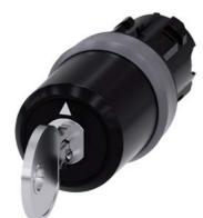
key-operated switch Siemens, 22 mm, round, plastic with metal front ring, lock number SSG10, with 2 keys, 3 switch positions I-O-II, latching, actuating angle 2x45°, 10:30h/12h/13:30h, key removal O+I, with laser labeling, upper case
