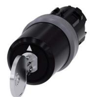
Key-operated switch BKS, 22 mm, round, plastic with metal front ring, special lock, with 2 keys, 3 switch positions I-O<II, latching on the left, momentary contact type on the right, actuating angle 2x45°, 10:30h/12h/13:30h, key removal O+I, Note: BKS locking systems E1 - E25 supplied without key
