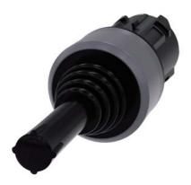
Coordinate switch, 22 mm, round, plastic with metal front ring, black, 4 switch positions, momentary contact type, without mechanical interlocking, with laser labeling, upper case and lower case, always upper case at the beginning of the word
